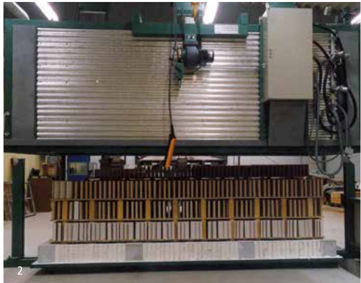
(1) Furnace hood with fibre insulation and meander-shaped heating elements (2) Hood furnace model HK 2000/12 with fibre insulation and meander-shaped heating elements
