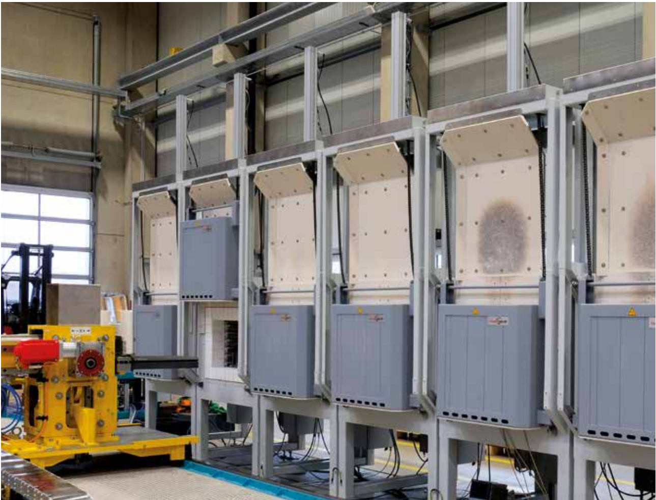
Plant with 6 chamber furnaces and linear traversing unit for charging
