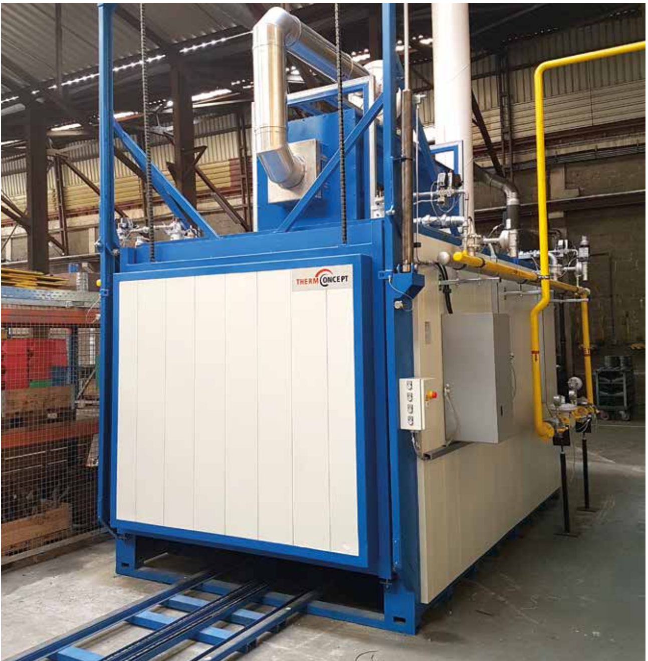
Gas-heated bogie hearth furnace with integrated thermal afterburner
