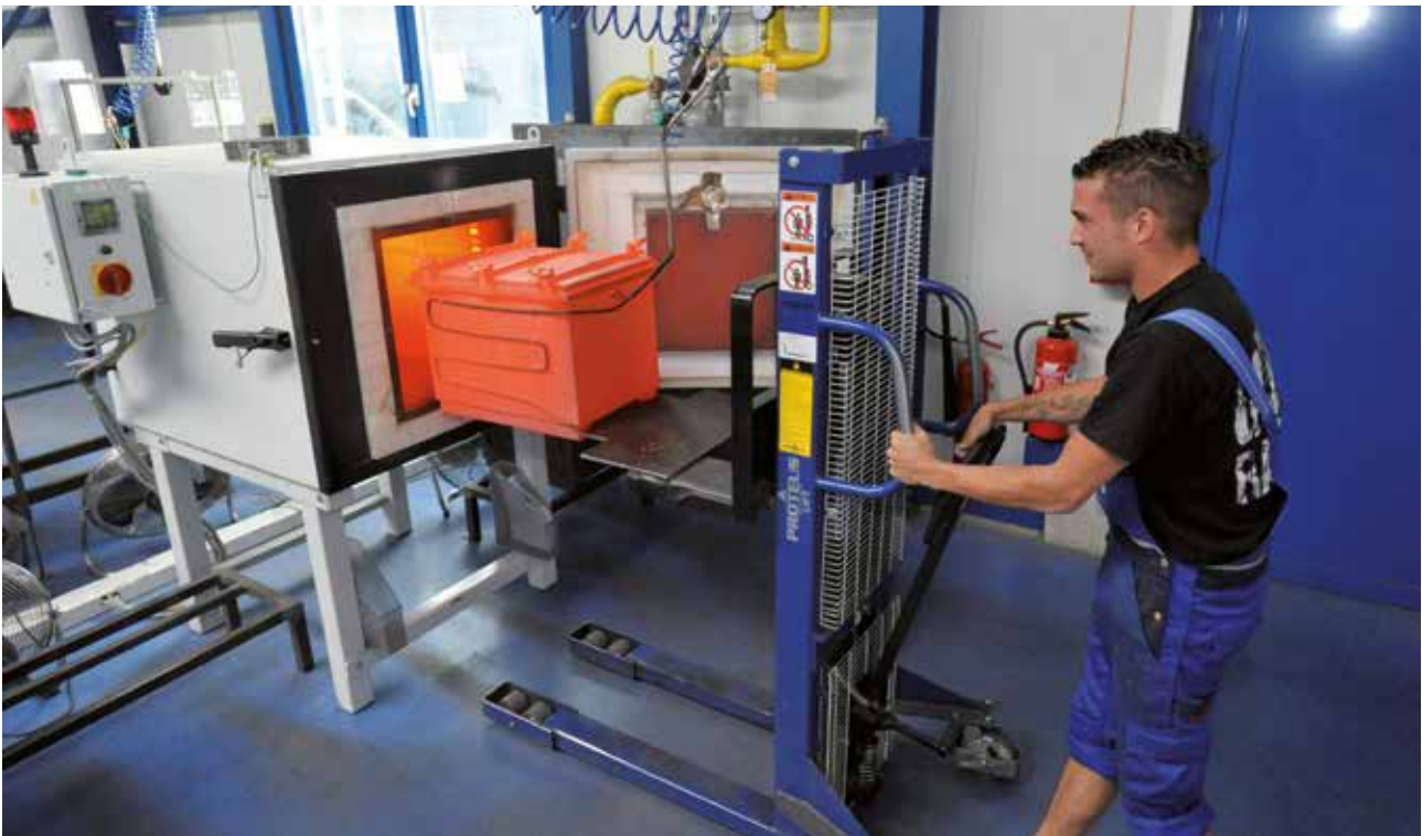
Air-circulation chamber furnace with gas box and fork-lift stacker
