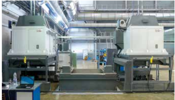
Fully automatic quenching and tempering system for aluminium components (solution annealing furnace, water bath, aging furnace)
