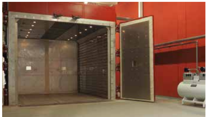
Electrically heated furnace plant (volume. 84m 3 ) for vacuum tempering of structural components for railway vehicles made from innovative composites
