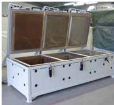
Shaft furnace with three separately controllable chambers for preheating steel rolls
