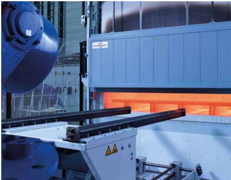
Preheating furnace with robot supported charging for press-hardening of sheet metals
