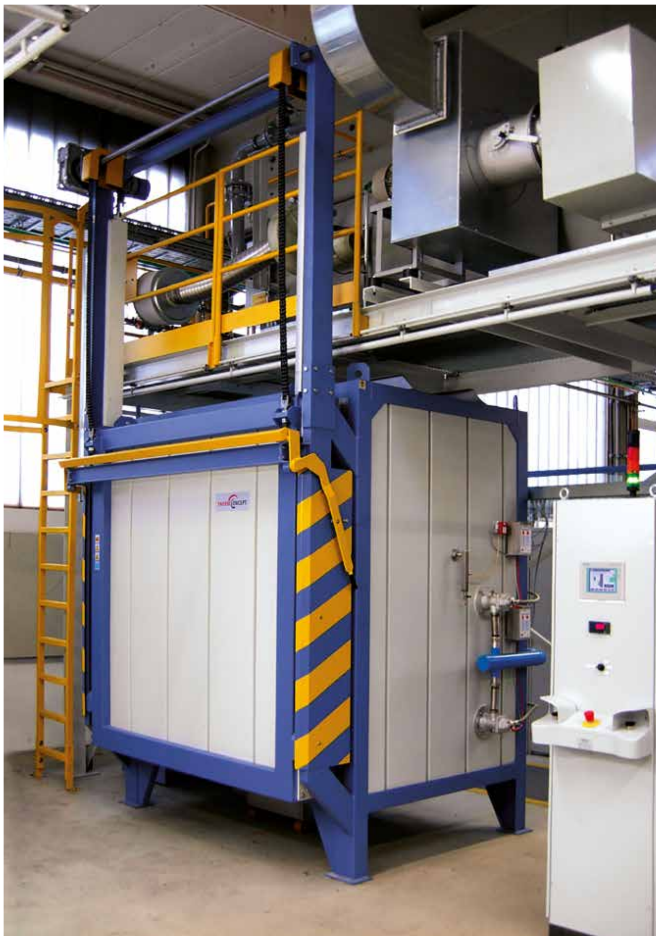
Gas-fired chamber furnace with integrated thermal afterburner for firing of lost wax moulds in turbine blade production
