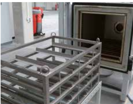
Air-circulation chamber furnace with gas box and fork-lift stacker
