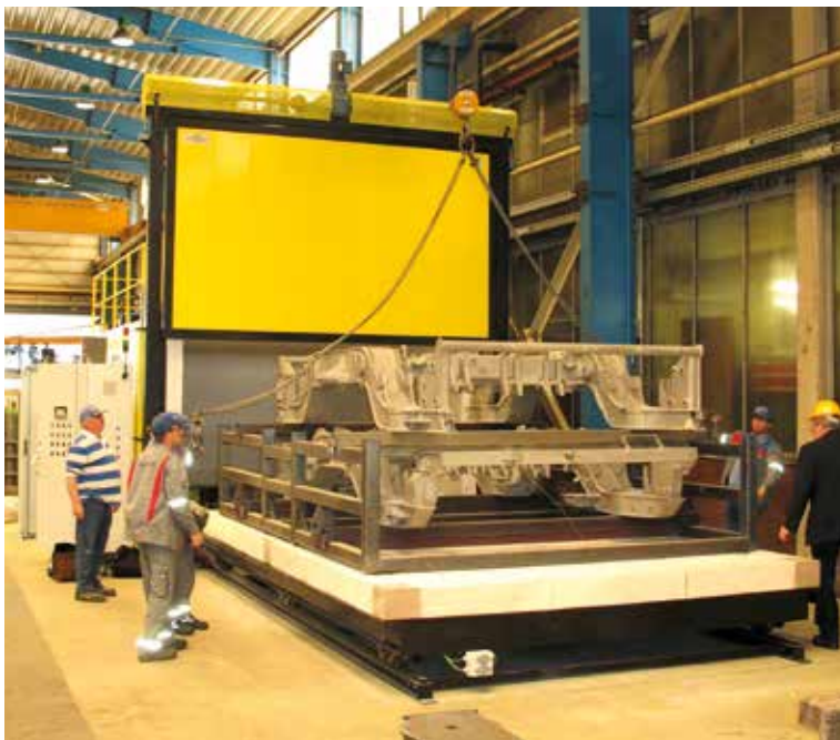
Gas-heated bogie hearth furnace for stress relieving of welded structures
