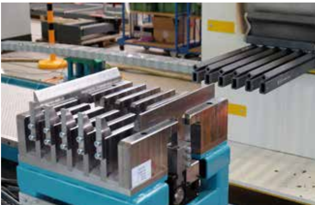
Hydraulic centering unit with suitable fork holder of the loading robot.
