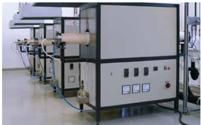
Production line consisting of 4 high-temperature tube furnaces for de-binding and sintering of ceramics after 3D printing
