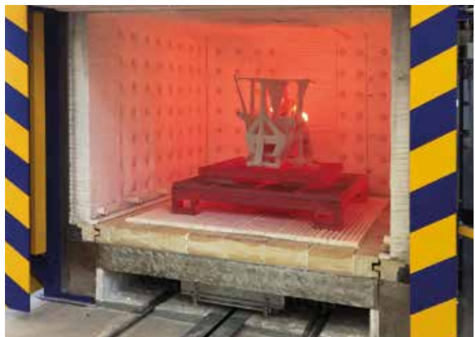
Gas-fired bogie hearth furnace for de-waxing and firing of investment casting moulds, with integrated thermal post-combustion
