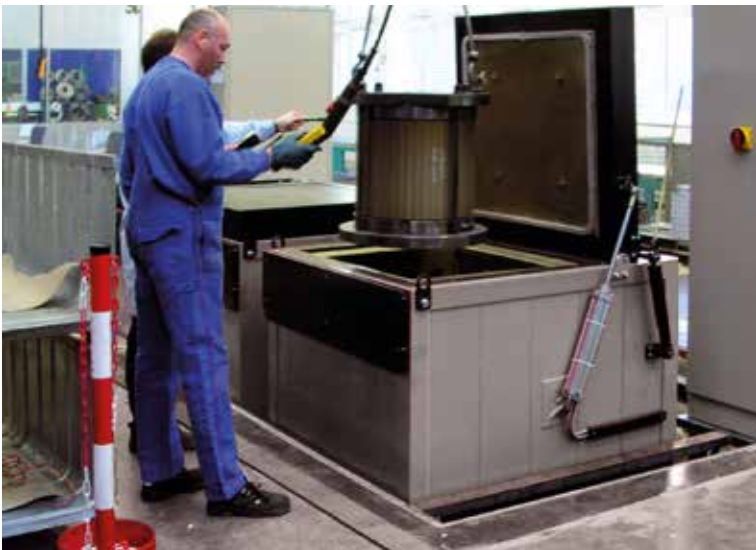
Model SM 1000/06/HA consisting of four shaft furnaces for heat treatment of machine parts
